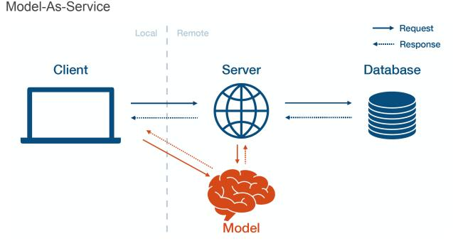
Model-as-service means that you deploy the model separately as its own service. The client and server can interact with the model by making requests to the model service and receiving responses.
