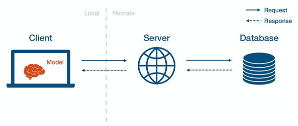
Edge prediction means that you first send the model weights to the client edge device. Then, the client loads the model and interacts with it directly.
