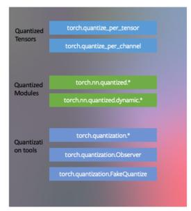
Model quantization is a model compression technique that makes the model physically smaller to save disk space and require less memory during computation to run faster. It decreases the numerical precision of a model's weights. In other words, each weight is permanently encoded using fewer bits. Note here that **there are tradeoffs with accuracy**.
